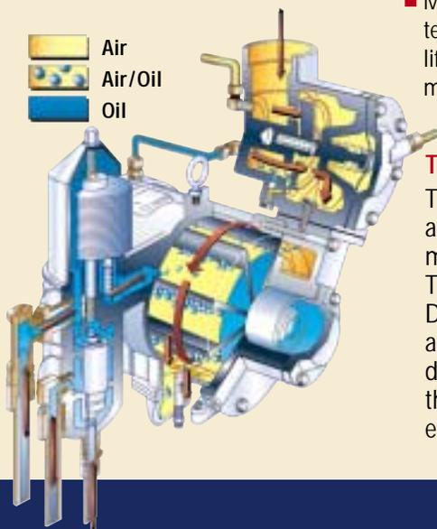
**The Perma-Vane® Air End Principle**
